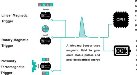
Pulse energy can be harvested to generate power for electronic circuits. Wiegand sensors can additionally serve as part of a wireless power transmission system
