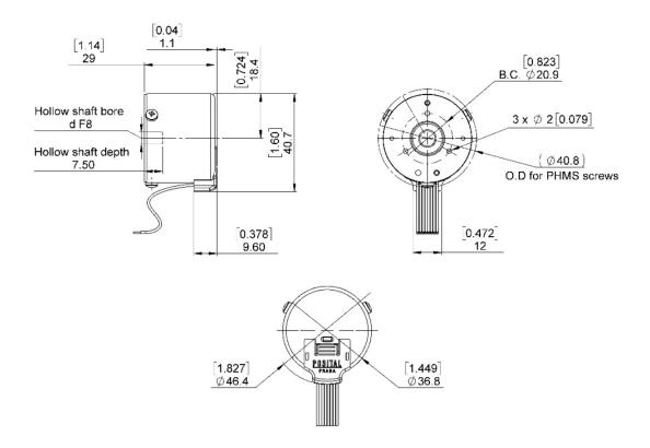
E6xU-PRQ: d = Ø4mm, Ø5mm, Ø6mm or Ø1/4"
