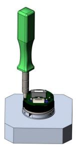
Tighten the two M2 screws using a Torx T6 key with a torque of 0.25 Nm.
