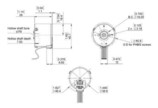
E5xU-PRQ: d = Ø4mm, Ø5mm, Ø6mm or Ø1/4"
