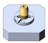
Tighten mounting screws while pushing down on the centering tool and remove centering tool. Tighten screw to a typical torque of 0.4 Nm (Actual torque value may change due to machine screw selected and base mounting material)
