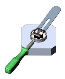
Tighten both set screws with a 1.3mm [0.05"] hex key, using the channel hole in the adapter plate with a torque of 0.5 Nm.
