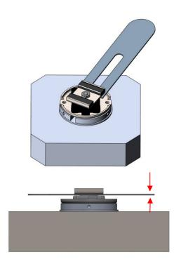
Slide gapping tool (Required thickness of 0.7mm [0.0275"]) between magnet and plastic frame on the bottom shield. Push magnet down.
