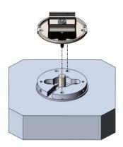
Screw the two Socket Set screws into the Magnet-Hub-Assembly to secure. Make sure that the screws do not enter the inner side of the Magnet-Hub-Assembly.
