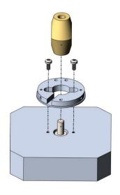
Slip adapter plate over shaft and use screws, depending on tapped holes in motor frame, to secure. Slip centering tool over shaft to center adapter plate to the shaft centerline.
