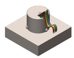
Connect cable assembly to the PCB by plugging the connector into the PCB.
