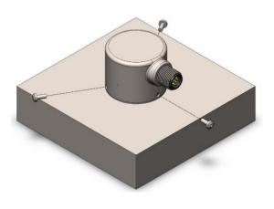
Secure housing by tightening the three M2.5 screws using a Philips screw driver with a torque of 0.4 Nm
