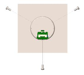
Slide housing over adapter plate. Secure housing by tightening the three M2.5 screws using a Philips screw driver with a torque of 0.4 Nm
