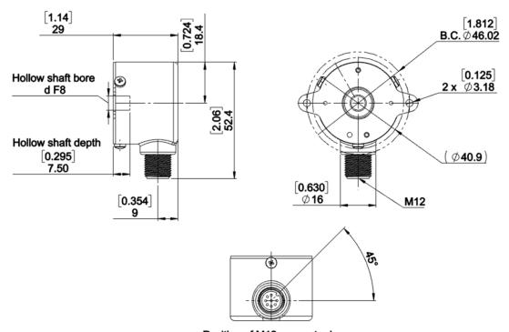
Position of M12 connector key
