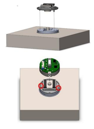
Slide bottom shield/magnet assembly over shaft and lock alignment pins into adapter plate. Push down bottom shield all the way so it lies flat on the adapter plate.
