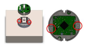
Align PCB with carrier to frame (two different keys) and push down until it locks into place.
