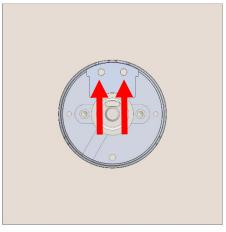
For a correct flange orientation, notice the two holes shown in the image. The connector location should be always assembled relative to these two holes.
