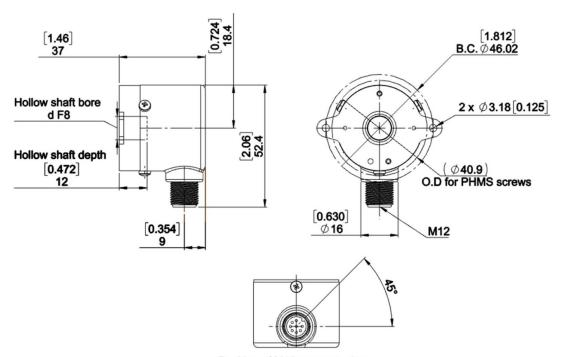
Position of M12 connector key
