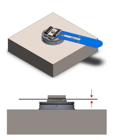
Slide gapping tool (Required thickness of 0.7mm [0.0275"]) between magnet and bottom shield. Push magnet down.
