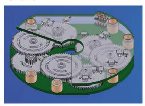
Linear systems normally need more than one turn of a shaft. A single turn encoder is unsuitable for this type of application because of the additional requirement of the number of turns. The principle is relatively simple: Several single turn encoders are connected using a reduction gear. The first stage supplies the resolution per turn, the stages behind supply the number of turns. In the following picture you can see the gearing module with the several stages of reduction gears.
